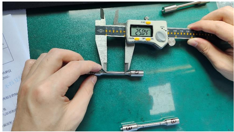
Figure 4 L_0 length Marking
