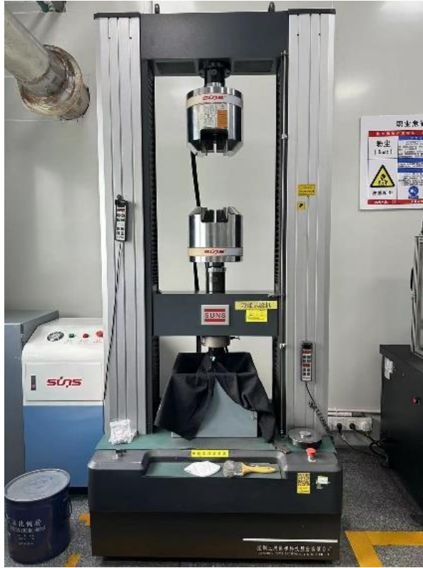
Figure 7 SUNS microcomputer controlled electronic universal testing machine
